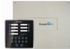
The unit is a fixed S8 programming control panel with 7 alarm inputs and one reserved tamper function input. The 7 zones/entrances are divided into 2 areas. “Entrance time” and “exit time” function, connections for up to 8 key insertion units and 8 SimplyTouch keypads (30010102). Self-powered siren output, internal siren output, voltage free alarm output, 4 open-collector outputs for miscellaneous signals (battery status, system status, etc...). Alarm memory available via SimplyTouch keypad.
