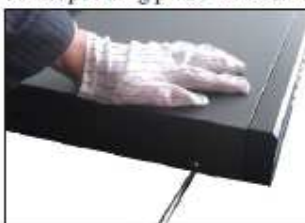
6. Fix the screws of the top cover .
