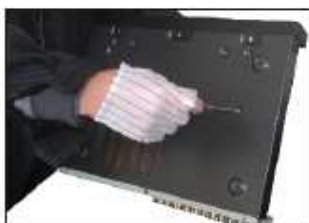
5. Fix the screws of the hard disk.
