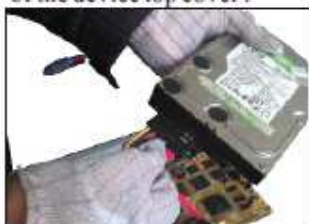
3. Connect hard disk power line
